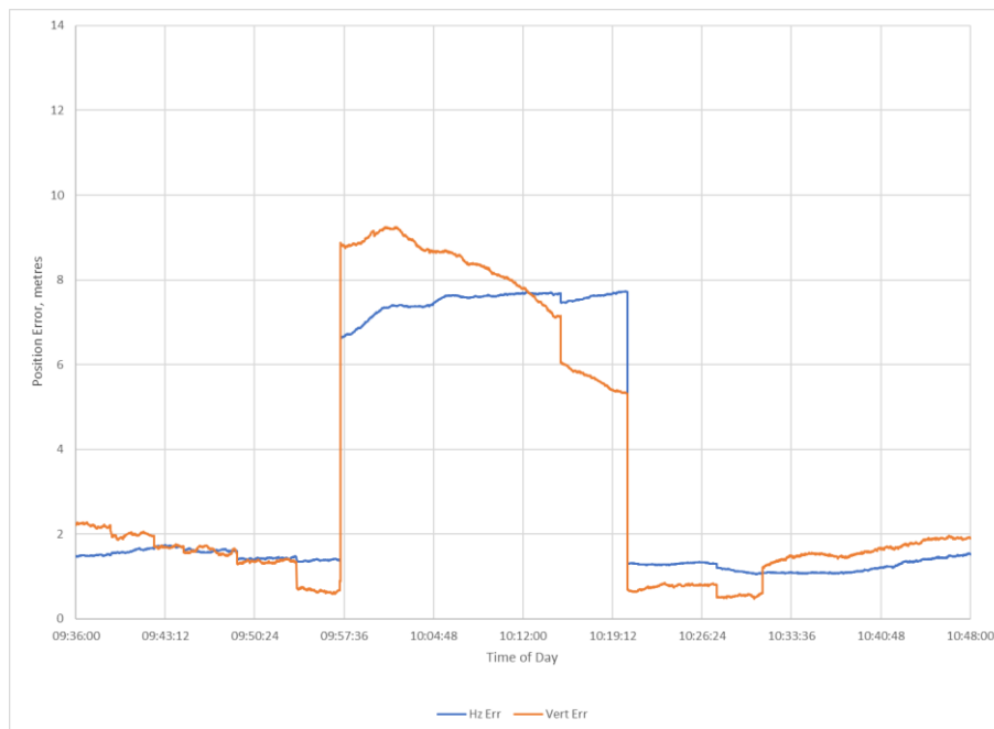
Figure 5-2: Position Error during period of High PRN01 Error on 10 th July 2023 at SLGO
