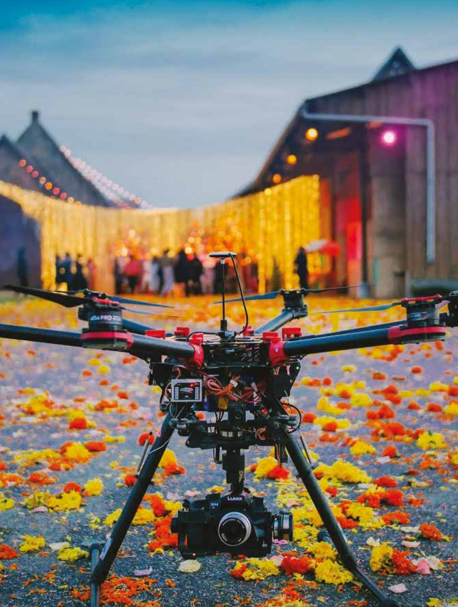
Over 6,300 drones have been registered with the IAA. This one has been fitted with a gyro stabilised aerial camera so that it may be used for aerial photography and cinematography. Image supplied by Aerial Photography Ireland.
