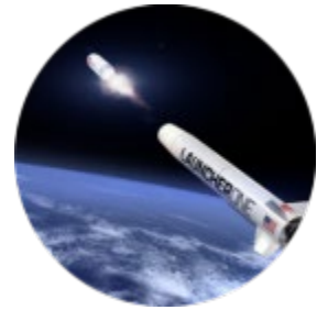
First and Second Stage Separation
