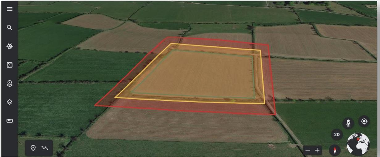
**Step 7.** The pilot's position is to be added as a placemark (*New Item*). The same process is repeated with the UAS take-off and
