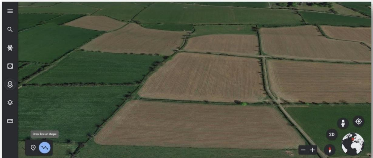
**Step 3.** Lines are drawn as the outer contour of the Flight Geography. Click to create a corner point. The coordinates of these corner points (here in the picture small circles) are saved later in the \*.kml file. The contour is closed by clicking on the starting point.
