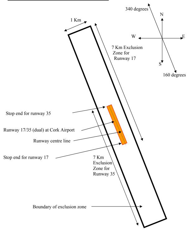
Note 1 All bearings are given in degrees **east of True North** Note 2 This diagram is not to scale
