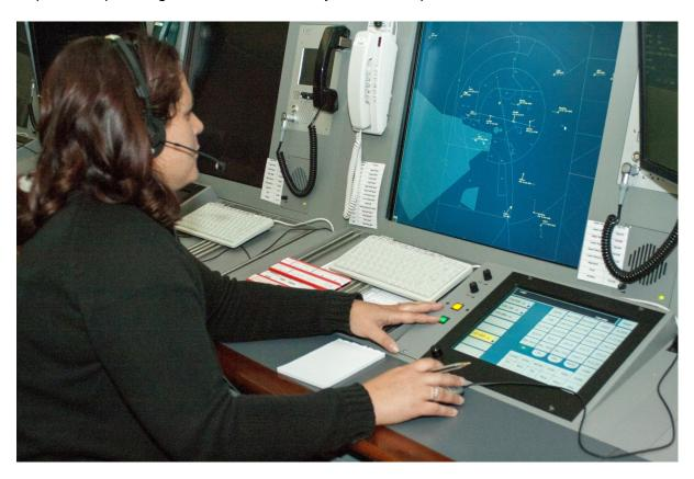
Controllers use a touch-screen Voice Switching and Communications System to coordinate flights with other controllers.
