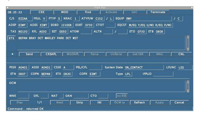
The ATC Eurocat flight plan window contains the flight plan details for an individual flight, including the SSR code which is automatically allocated by the system. Creation of a flight plan using this window is a time-consuming and complex process.
