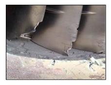
The photographs above highlight the significant damage caused to parts of an aircraft as a result of a bird strike incident.
