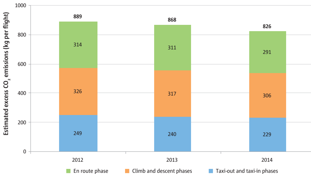
Figure 4.4 Estimated excess CO 2 emissions per flight are decreasing in taxi, take-off, climb/descent and en route phases 26
