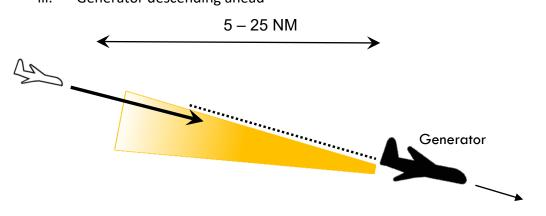
Note: The variability in the generator aeroplane rate of climb or descent makes it quite difficult to estimate exactly where the vortex is. Consequently, during the en-route phase of flight, Pilots should expect possible wake encounters when other traffics in proximity appear to be on similar tracks ahead, crossing above your level, climbing or descending ahead through your flight path, while wind direction is likely to move the wake towards your trajectory.
