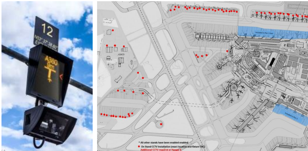
Figure 8.4: A-VDGS and Stand CCTV camera installation (indicative)
