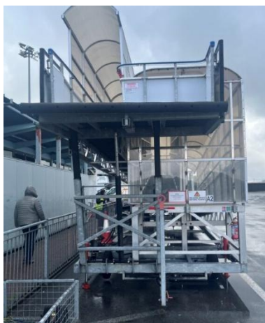
Figure 7 Aviramp - ramp used for accessing aircraft
