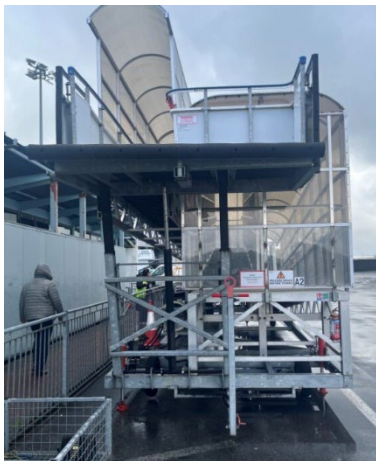
Figure 10: Aviramp - ramp used for accessing aircraft
