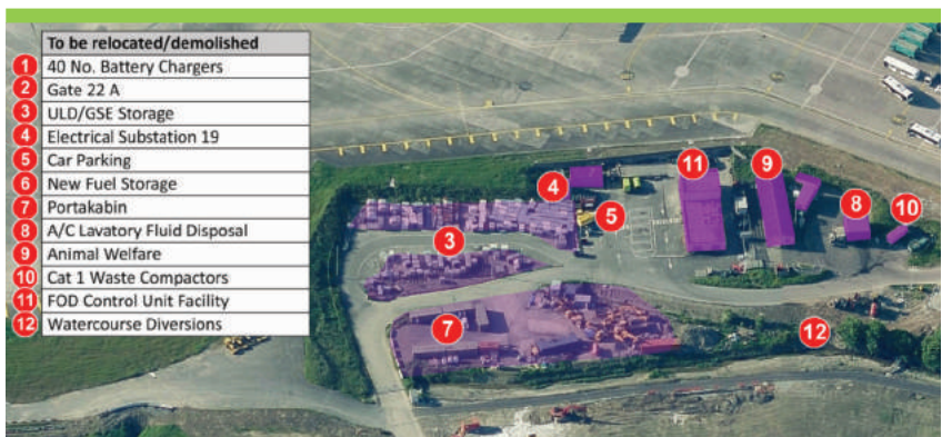
Required relocation of existing facilities on footprint of proposed South Apron Stands phase 2 site.
