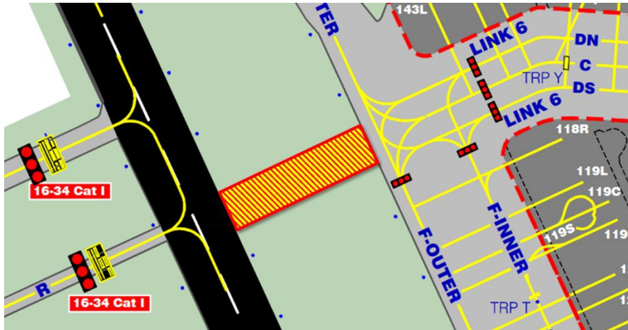
Figure 12: Taxiway joining Link 6 and Runway 16-34
