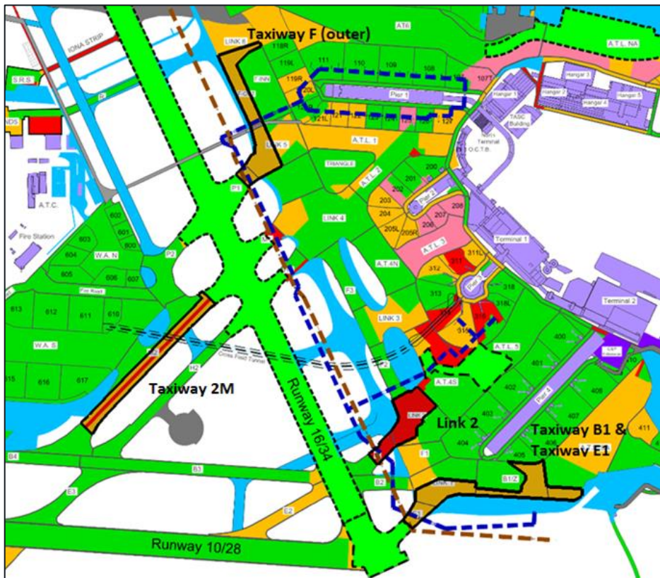
Figure 4.3: Airfield Taxiway Rehabilitation Programme
