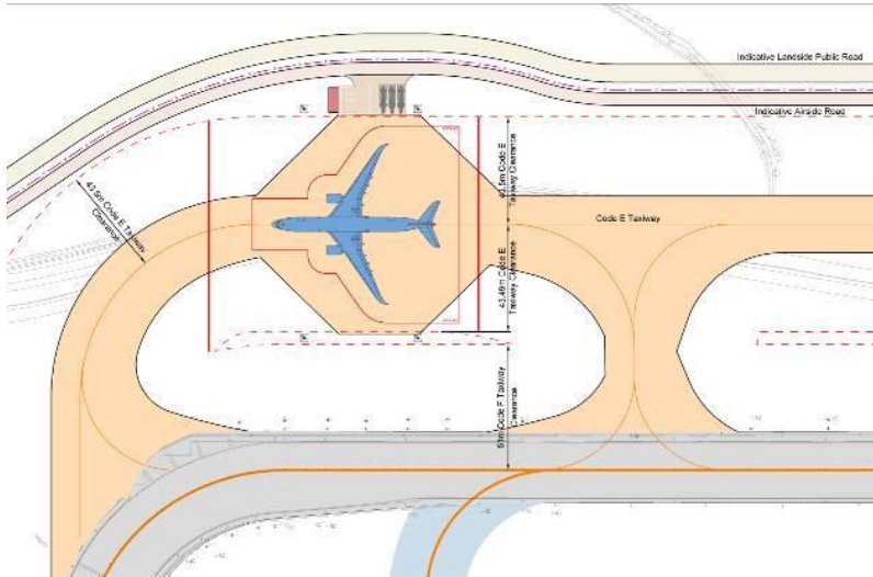
Figure 6.23: De-Icing Pad at Runway 10R
