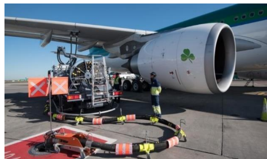
Exhibit 6.42 – Example of Hydrant Fuelling
