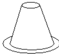
Figure 6.4 Conical marker for grass runways and taxiways
