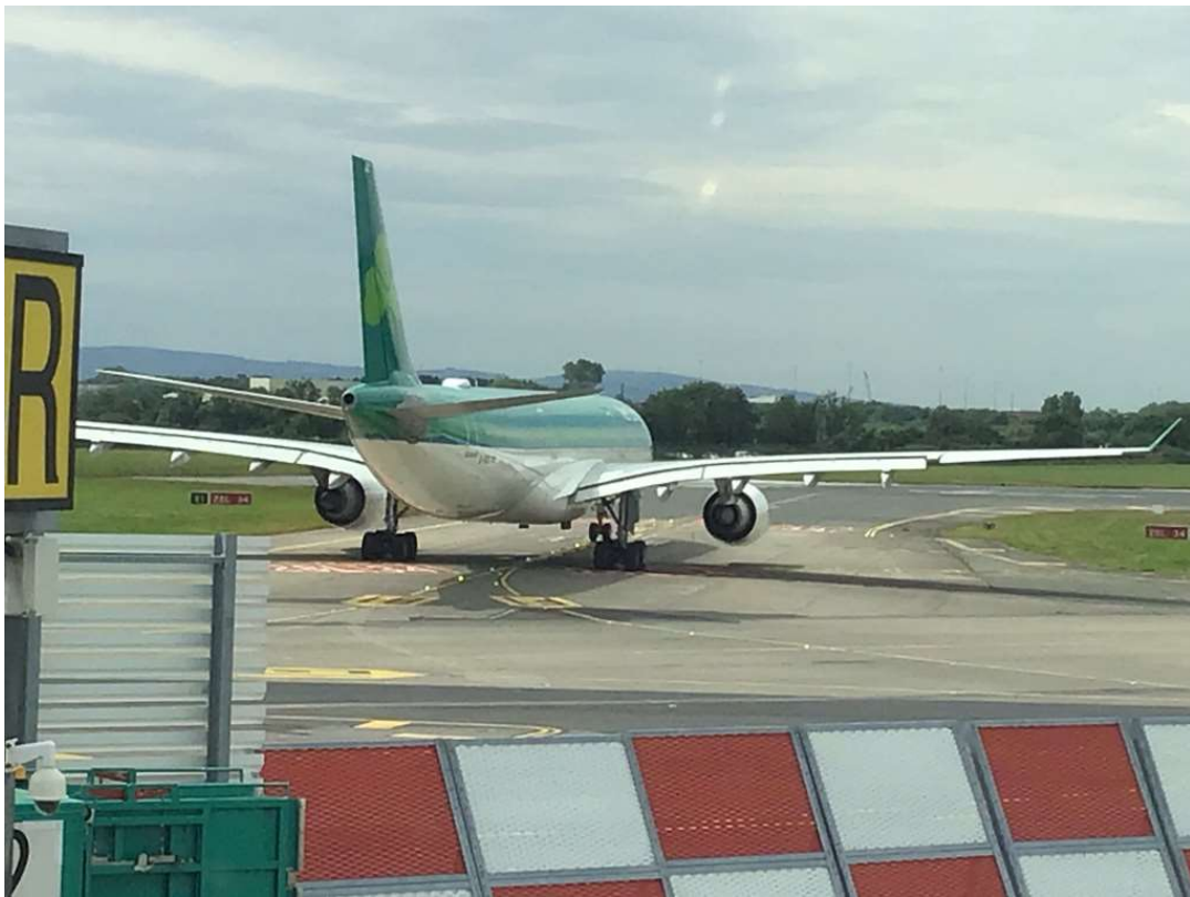
Fig 3: An A330-300 holding on taxiway E1 short of the existing CAT 1 hold.
