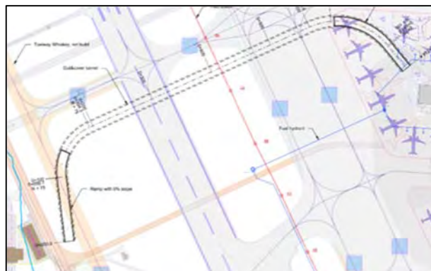
Figure 101: Underpass Location – Off Pier 1
