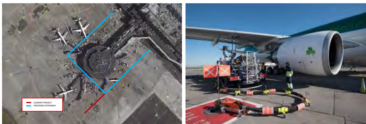
Exhibit 1. Left to right: Plan view of proposed fuel extension around Pier 3 and photo of fuel hydrant.
